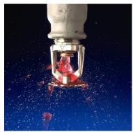
2- Heat expands the liquid, the air is compressed and the glass shatters
