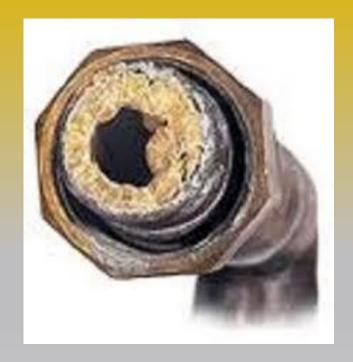
A Badly Limescale damaged valve restricting flow of water into boiler
