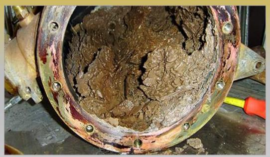
This is scale inside a coffee boiler that built up over a period of 9 months (it doesn't affect coffee though as that is filtered)
