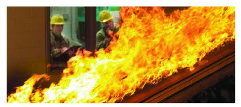
These are large scale tests using a re-entrant corner (as per BRE testing).
