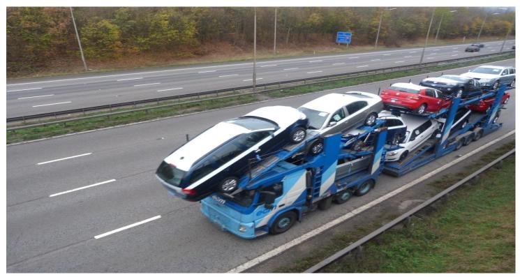
Eleven cars are being carried! Loading and unloading is done by the driver. In some locations the cars will be driven short distances on the public highway
